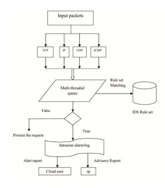
Figure 3: Data flow diagram of proposed multi threaded intrusion detection model
